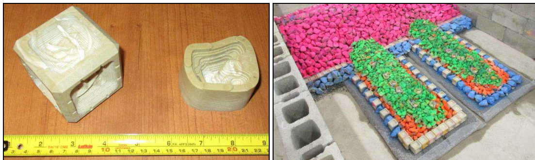
Figure 5. Model scale EConcrete® units fabricated and tested during this study.
