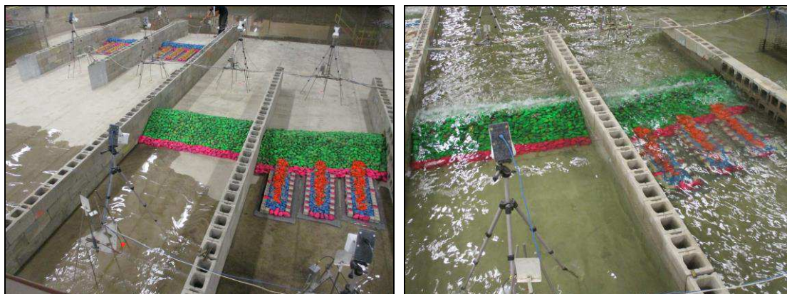
Figure 6. Breakwater model setup and testing for Test Series A.
